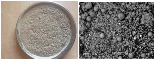
Fig. 1: The Original Picture and SEM Picture of Fly Ash [8].
